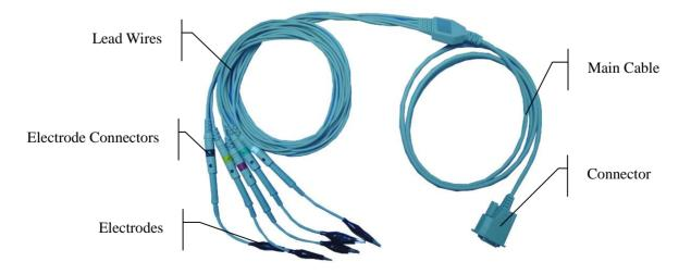
**Connecting Main Cable:** Plug the connector of main cable into the patient cable socket on the right side of the unit, and secure the screw.
