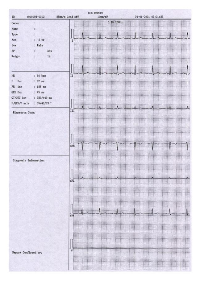
As figure above shows, the USBPRT mode record includes: ID, Record speed, Hint information, Sensitivity, Date and time; Owner, Name, Type, Age, Sex, BP, Weight; Heart Rate, P duration, PR interval, QRS duration, QT/QTC interval, P/QRS/T axis; Minnesota code; (Written by doctor) Diagnosis information; (Written by doctor) Report confirmed by; (Written by doctor) ECG waveform of 7 leads;
